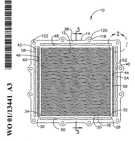
(57) Abstract: A fuel cell bipolar plate including a plurality of reactant channels (18, 24) defining respective inlets and outlets and at least two flow restrictors (54, 56) respectively associated with at least two adjacent reactant channels.
